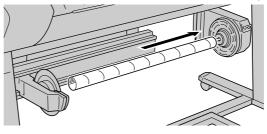
**5** With your left hand, push the slide holder toward the left end of the media core, and continue to push firmly until you hear the hub of the slide holder catch and lock into the core media.
